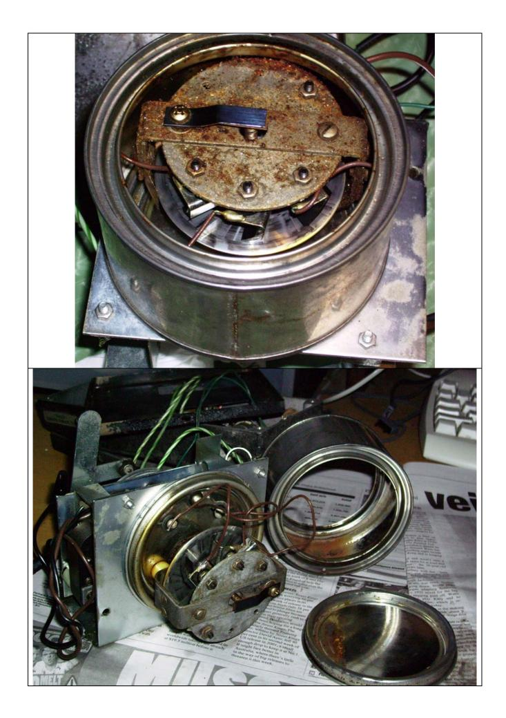
Operation with 110VAC 50Hz showed that motor worked, and power supply rails showed 67VDC and 13VDC, with the secondary (two red wires) at 46.7VAC unloaded. The transformer white wire is from a screen, and is soldered to the ground.
